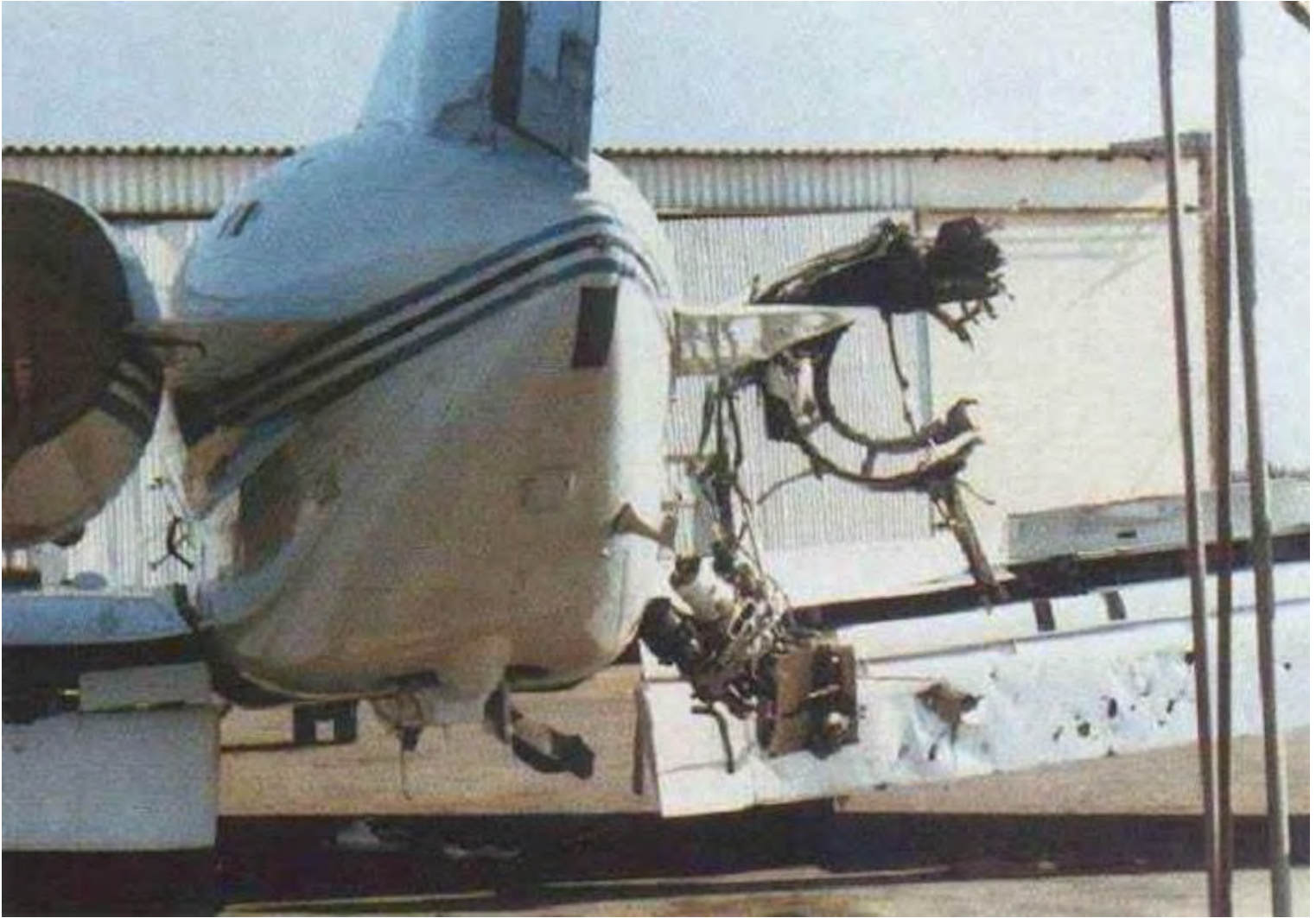
VIP BAe 125-800 after missile strike to right engine in 1988. Credit: Aviation Week
