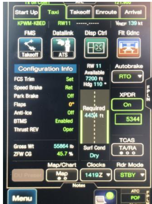
A Gulfstream GVII taxi "Phase of Flight" page with one item missing.
