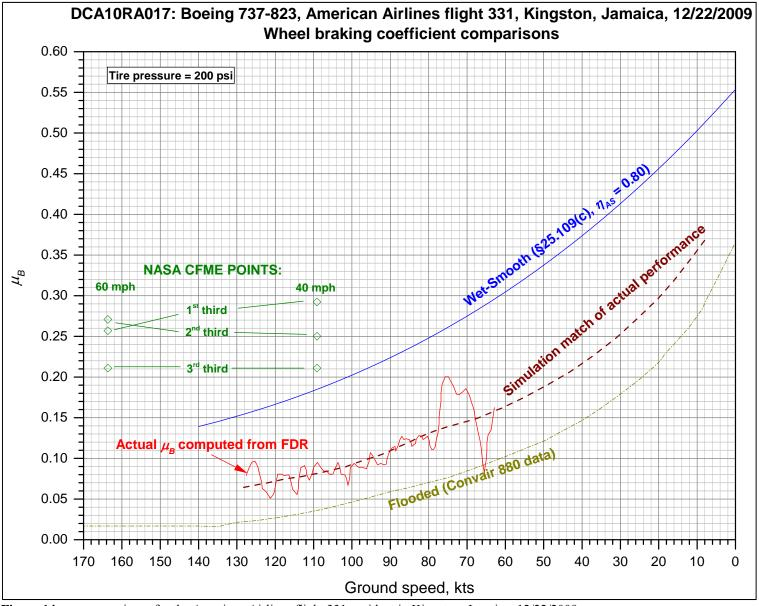
**Figure 14.**  $\mu_B$  comparisons for the American Airlines flight 331 accident in Kingston, Jamaica, 12/22/2009.
