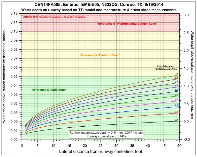
Figure 19. Water depth calculations for the EMB-505 (N332QS) accident in Conroe, TX, 09/19/2014.
