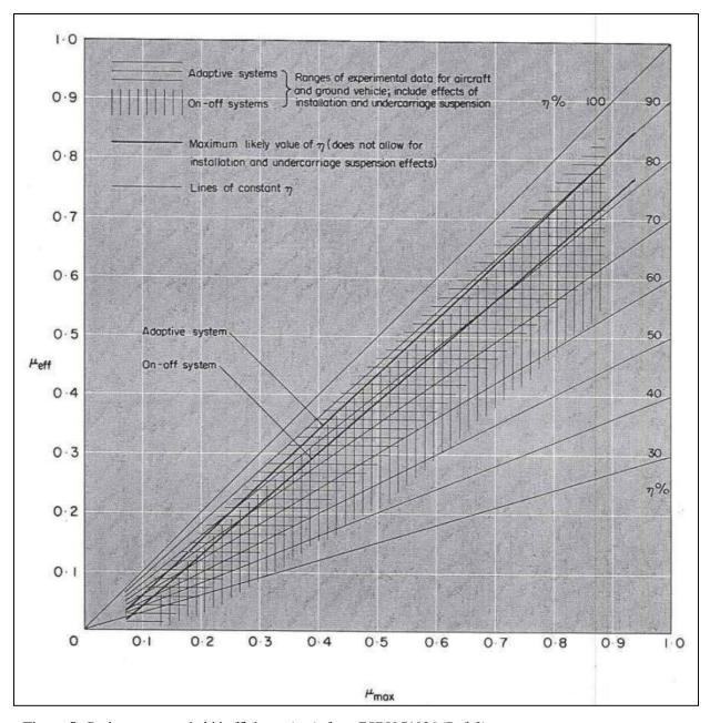
**Figure 5.** Brake system anti-skid efficiency ( $\eta_{AS}$ ), from ESDU 71026 (Ref. 2).
