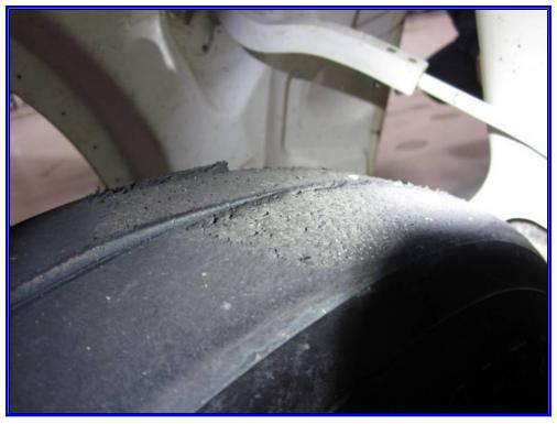
**Figure 11b.** Post-accident photo of N584JS left main gear tire, showing evidence of reverted-rubber hydroplaning (photo of right tire not available).
