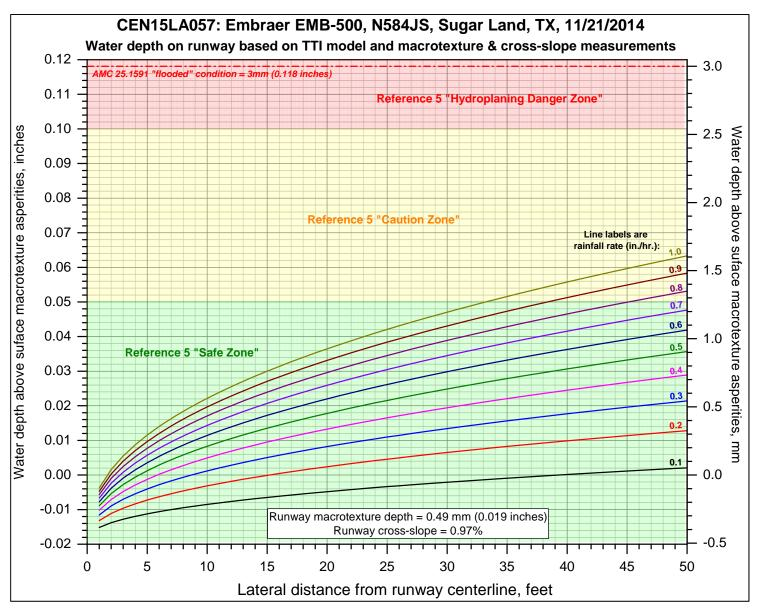
**Figure 21.** Water depth calculations for the EMB-500 (N584JS) accident in Sugar Land, TX, 11/21/2014.
