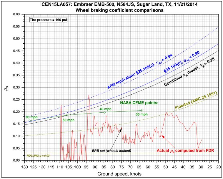
**Figure 20.**  $\mu_B$  comparisons for the EMB-500 (N584JS) accident in Sugar Land, TX, 11/21/2014.
