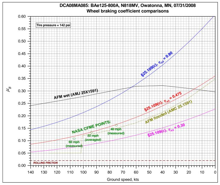
**Figure 12.**  $\mu_B$  comparisons for the BAe 125-800A (N818MV) accident in Owatonna, MN, 7/31/2008.
