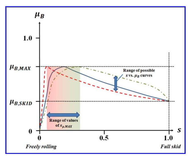
**Figure 2.** Plot of  $\mu_B$  vs. s (adapted from Ref. 2).
