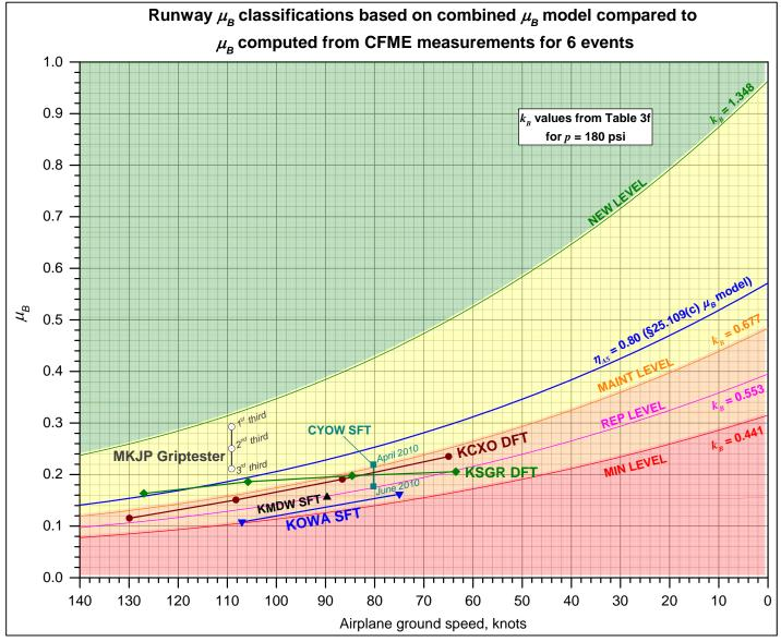
**Figure 25.** Runway  $\mu_B$  classifications based on CMB model, compared to  $\mu_B$  from CFME measurements.
