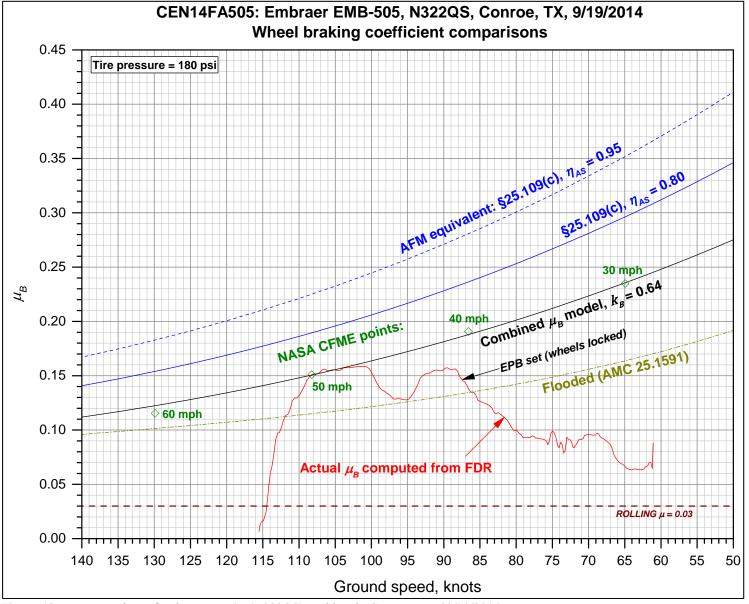
**Figure 18.**  $\mu_B$  comparisons for the EMB-505 (N322QS) accident in Conroe, TX, 09/19/2014.
