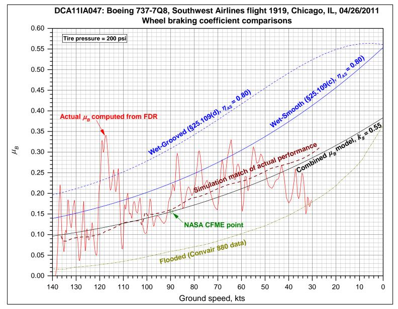
**Figure 16.**  $\mu_B$  comparisons for the Southwest Airlines flight 1919 incident in Chicago, IL, 04/26/2011.
