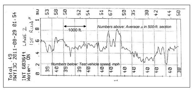
Figure 17a. 40 mph SFT run on KMDW runway 13C, 10 ft. left of centerline (from Ref. 21).
