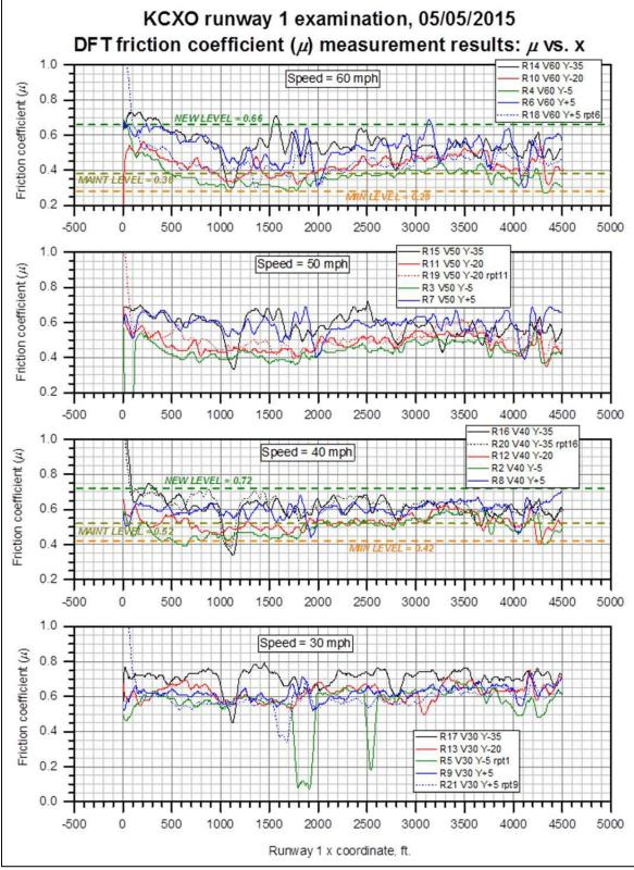
**Figure 23.** DFT measurements on KCXO runway 1. The runway coordinate system origin as at the threshold; x is down the runway centerline, y is to the right of the runway centerline. Legend entries indicate run number (R), DFT speed in mph (V), and runway y coordinate in ft. (Y).
