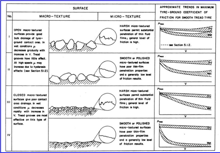
**Figure 3.** Effect of surface texture on  $\mu_B$ , from ESDU 71026 (Ref. 2).
