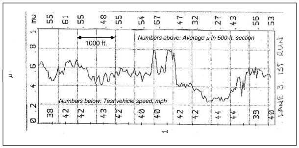
Figure 17b. 40 mph SFT run on KMDW runway 13C, 10 ft. right of centerline (from Ref. 21).
