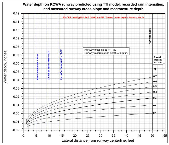
Figure 13. Water depth calculations for the BAe 125-800A (N818MV) accident in Owatonna, MN, 7/31/2008.
