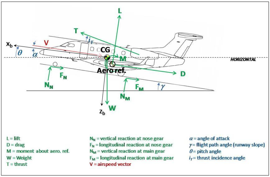
Figure 1. Free body diagram of forces on airplane during ground roll.
