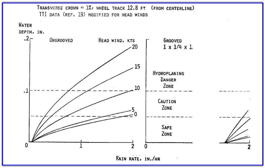
**Figure 4.** Runway hydroplaning potential during rainstorms, from Ref. 5.
