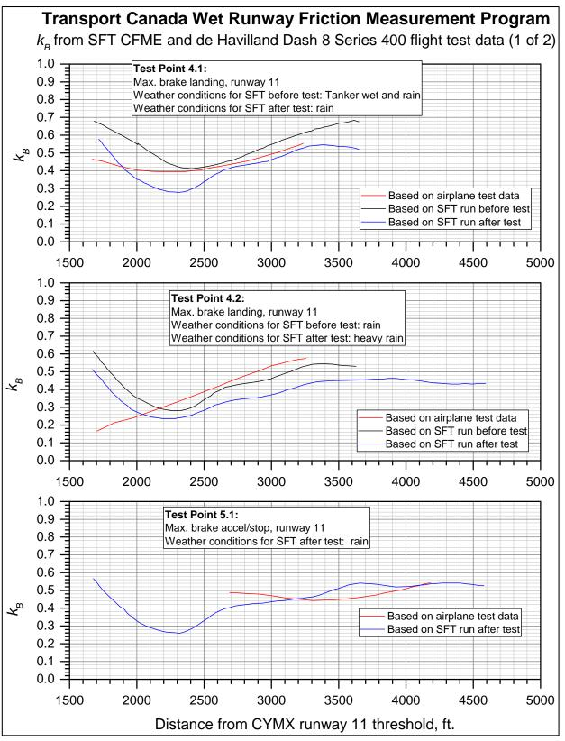
**Figure 26a.** Comparison of  $k_B$  computed from SFT measurements and DHC-8-400 flight test data (page 1 of 2).
