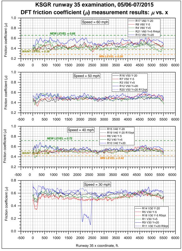
**Figure 24.** DFT measurements on KSGR runway 35. The runway coordinate system origin as at the threshold; x is down the runway centerline, y is to the right of the runway centerline. Legend entries indicate run number (R), DFT speed in mph (V), and runway y coordinate in ft. (Y).
