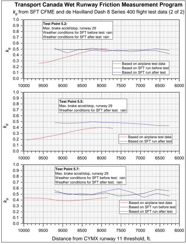
Figure 26b. Comparison of  $k_B$  computed from SFT measurements and DHC-8-400 flight test data (page 2 of 2).
