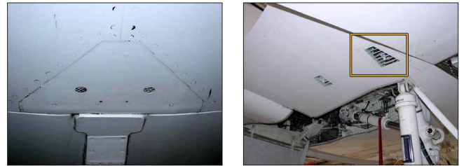
WING ANTI-ICE DUCTS THROUGH APU ACCESS PANEL (LOOKING INBOARD)
