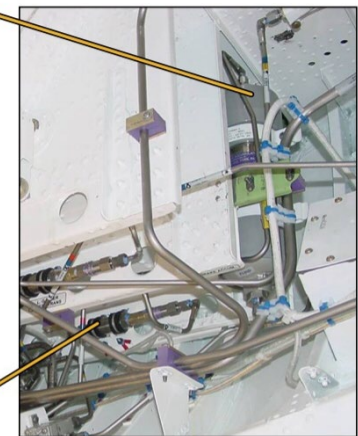
Park / Emergency Brake Pressure Gauge, Accumulator and Transducer
