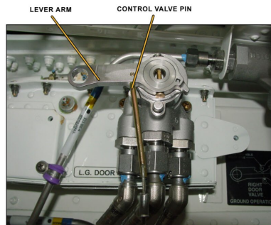
Main Landing Gear Door Control Valve Pin Installed
