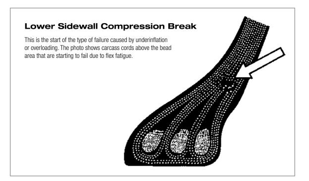
These photos show how underinflation or overloading can cause lower sidewall compression flex breaks.
