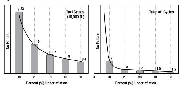
A couple of interesting findings in this study were that all the taxi cycle failures were blowouts in the lower sidewall, while the take-off cycle failures were thrown treads. From the shape of the curves we see that takeoff cycles were more sensitive to underinflation than were taxi cycles.
