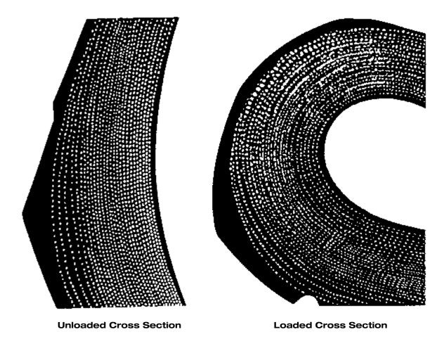
Tensile, compression and shear stresses can best be visualized by comparing an unloaded tire section to a loaded one as shown in the above photos. The following points can be made:
