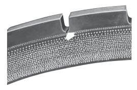
**Rib Undercutting** - is normally a continuation of the groove cracking that continues under the tread rib between the rubber and the tread reinforcing fabric
