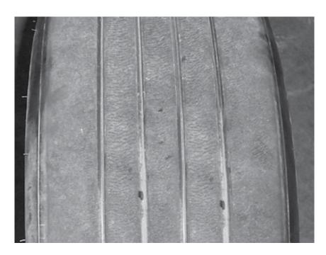
**Heavy Braking**Heavy braking can create a pattern of abrasion. This will wear normally during service. **Action:** None required.
