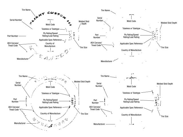
All Goodyear commercial aircraft tires are clearly marked with the following information: Goodyear, size, load rating, speed rating, molded skid depth, Goodyear part number, serial number, Goodyear plant identification and TSO marking. In addition, Goodyear tires are marked with the ply rating and other markings as required by airframe manufacturers or other organizations, such as an AEA code (which defines new tire casing and tread construction).
