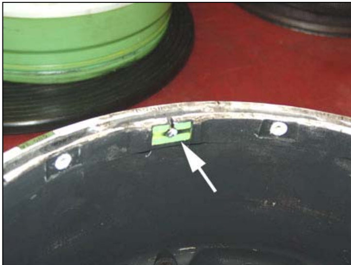
Area on wheel where an old style spacer was installed. Area with black strip is where cracking can occur.
