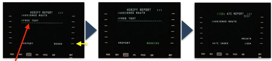
/ASSIGNED ROUTE element is a copy the Master FMS' Active Flight Plan (Downlink Message 40). Line-Select SEND.
