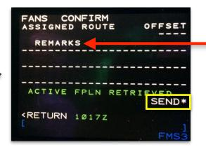
ACTIVE FPLN RETRIEVED automatically appears. Line-Select SEND\*. Downlink Message (DM40) is then sent to the Current Data Authority (CDA). NOTE: no REMARKS (Free Text) are necessary or recommended, as the objective of this message transaction is to mitigate transposition error.
