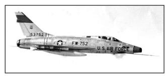
Examples in the Aerial Attack Study include references to the North American F-100 Super Sabre. This single-seat, single-engine jet aircraft was the first United States Air Force fighter capable of exceeding Mach 1 in level flight.
