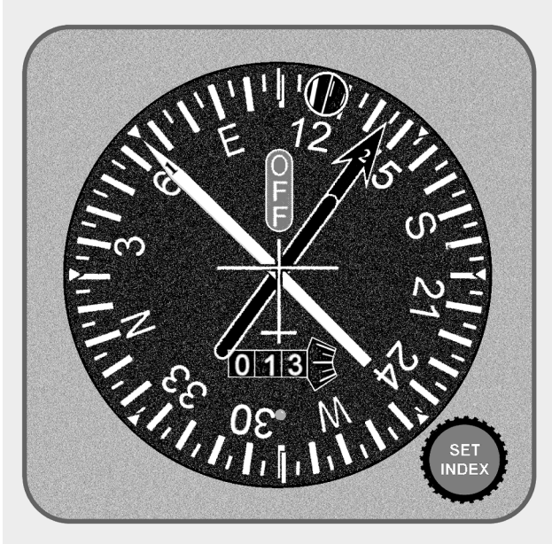
Figure 5.10. Bearing Distance Heading Indicator.
