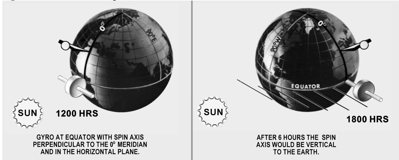
Figure 14.11. Direction of Spin Axis Affects Earth Rate Precession.
