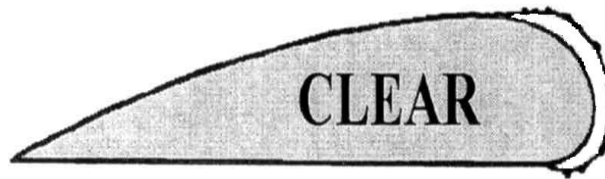
FIGURE 5. CLEAR ICE BUILDUP WITH HORNS
