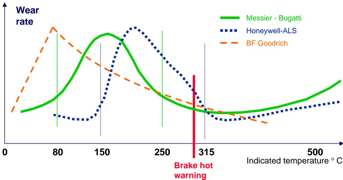
**Figure 6 - Carbon Wear vs. Indicated Brake Temperature
