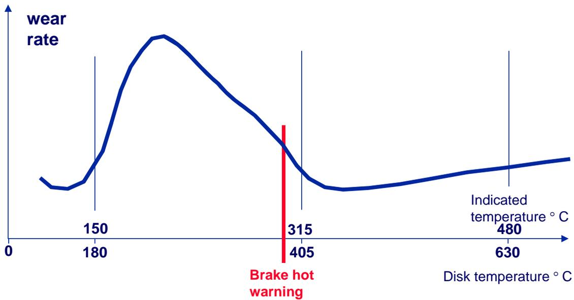
**Figure 3 - Carbon Wear vs. Brake Temperature according to HONEYWELL-ALS (A330 / A340)**
