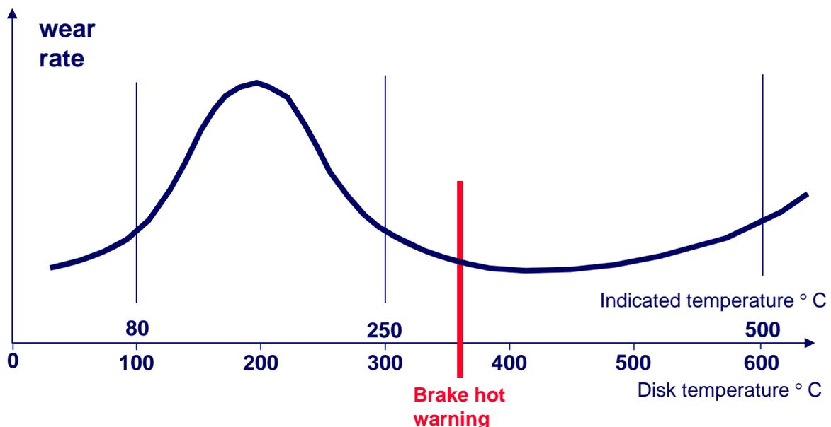
**Figure 2 - Typical Spectrum of Carbon Wear vs. Brake Temperature according to MESSIER-BUGATTI**
