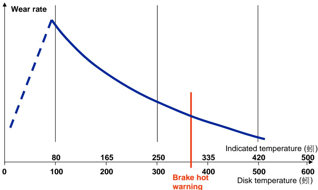
**Figure 4 - Carbon Wear Rates vs. Temperature according to BF GOODRICH (SUPERCARB - A321 / A330 / A340)**
