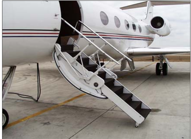
Main Entrance Door – Large-Cabin Gulfstream
