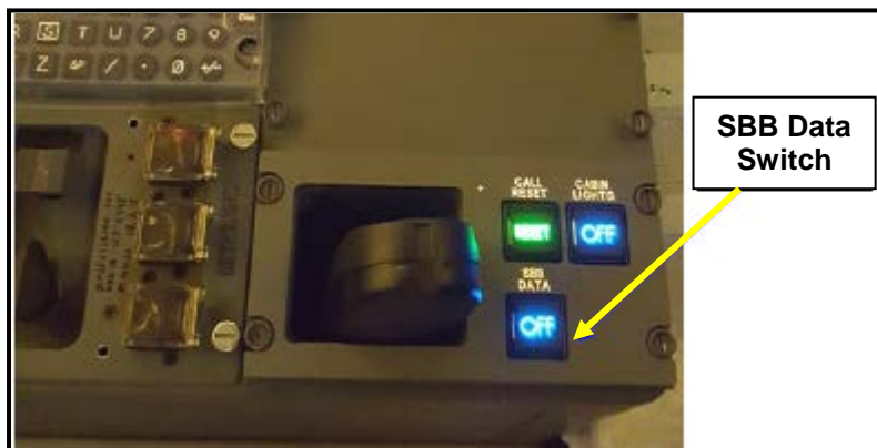
Figure 1 - Location of the SBB Switch in the Optional Switch Panel on the center pedestal
