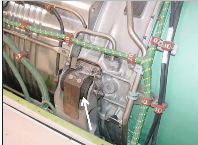
Arrow points to upper forward engine mount vibration isolator
