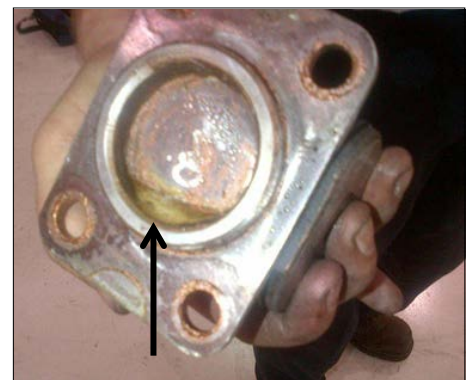
Water noted at forward engine mount after removal
