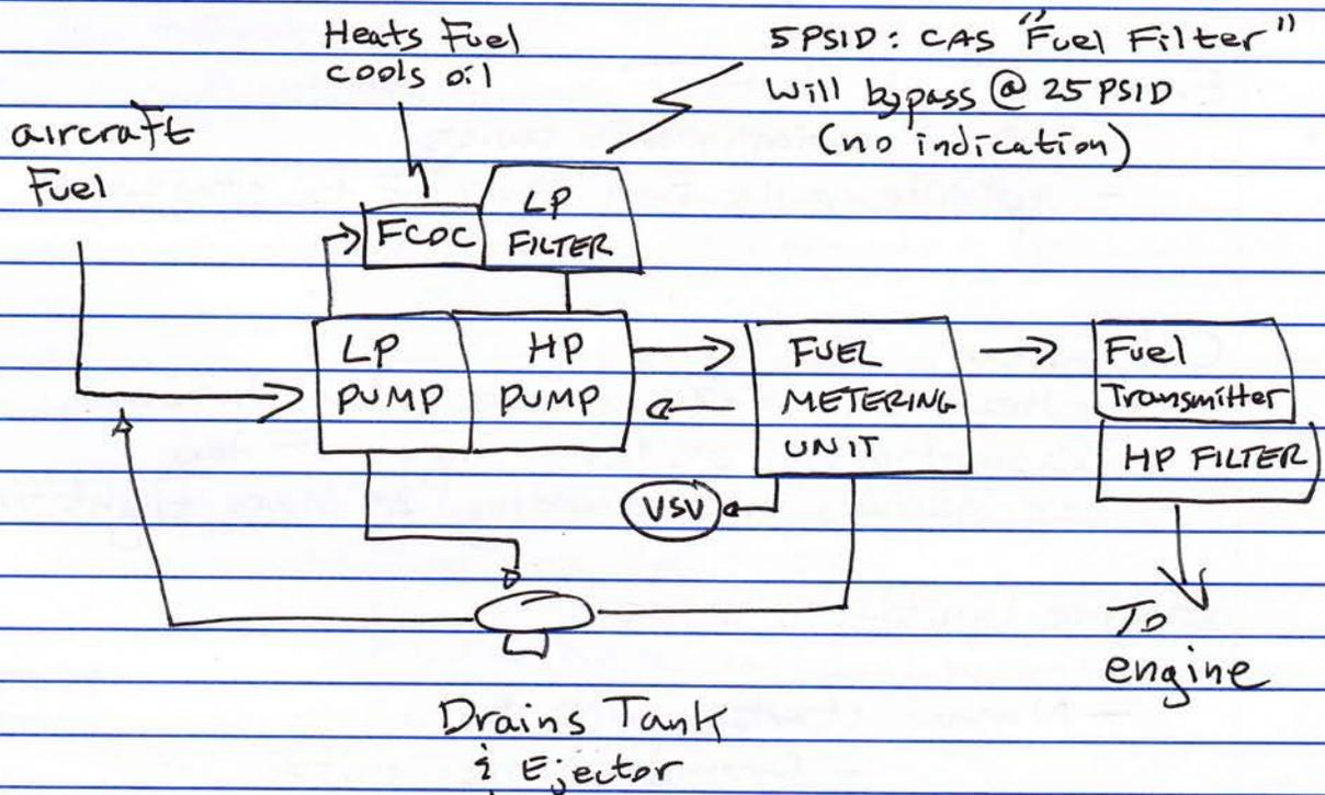
Variable Stator Vanes - First 3 stages of HP sends excess air to bypass to prevent compressor stalls
