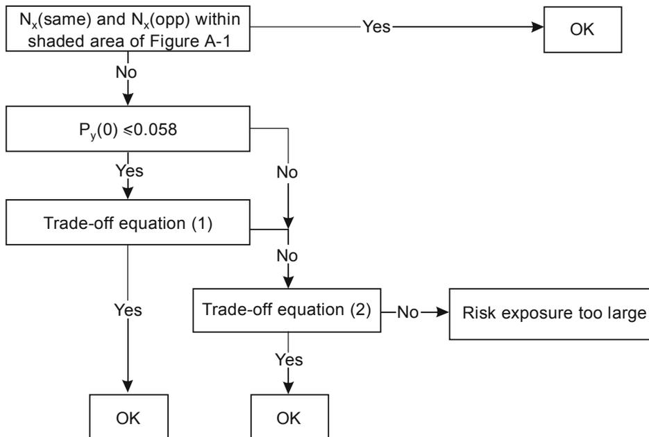
Figure A-2. Flow diagram of the trade-off between global system performance specification parameters for same- and opposite-direction traffic when  $P_y(0) \leq 0.058$  and on the assumption that  $P_z(1\ 000) \leq 1.7 \times 10^{-8}$
