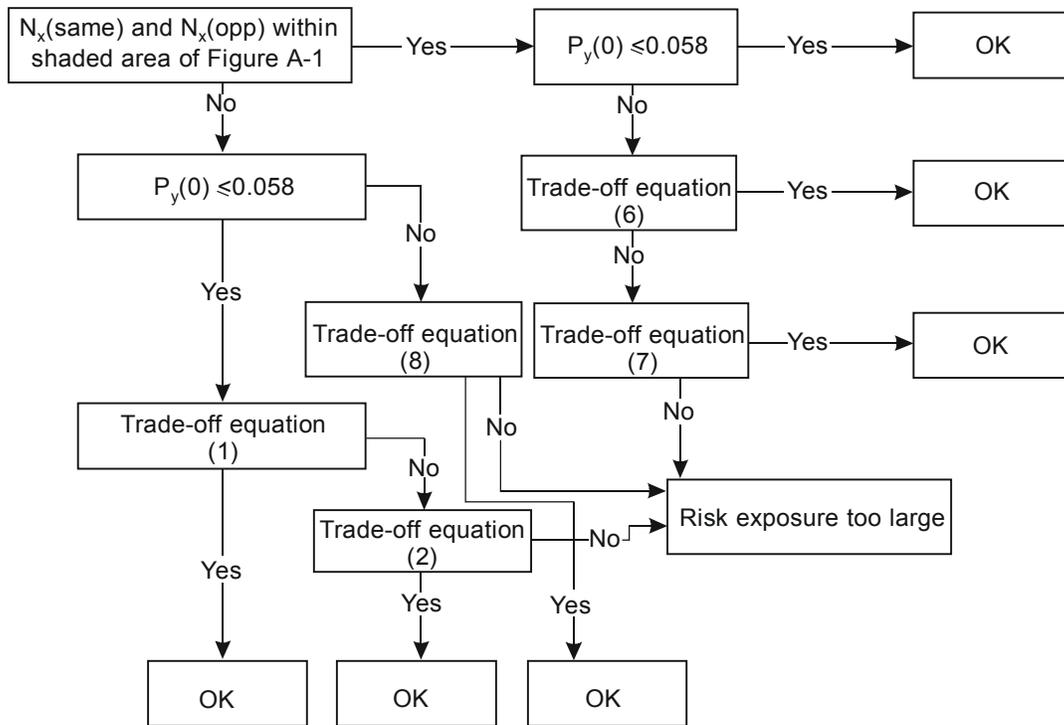
Figure A-5. Flow diagram of the trade-off between global system performance specification parameters for same- and opposite-direction traffic on the assumption that  $P_z(1\ 000) \leq 1.7 \times 10^{-8}$
