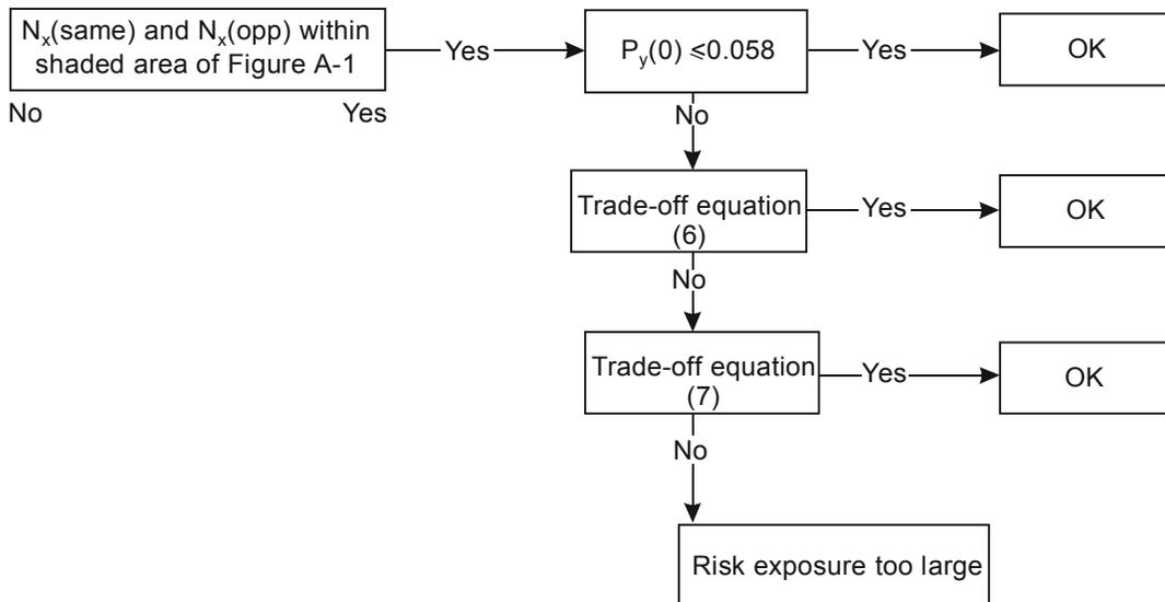
**Figure A-4. Flow diagram of the trade-off between global system performance specification parameters for same- and opposite-direction traffic when the combination of same- and opposite-direction passing frequency is within the shaded area of Figure A-1 and on the assumption that  $P_z(1\ 000) \leq 1.7 \times 10^{-8}$**
