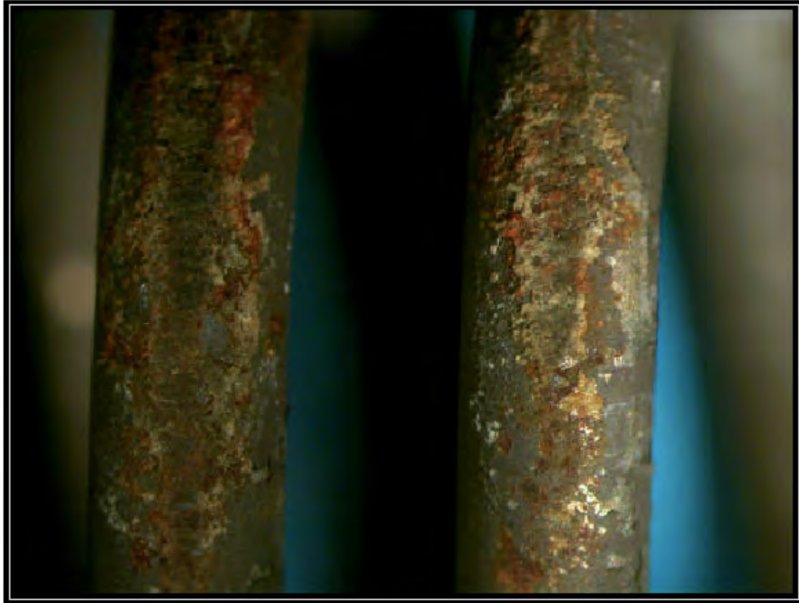
Figure 20: Photomicrograph of the corroded surfaces of the spring
