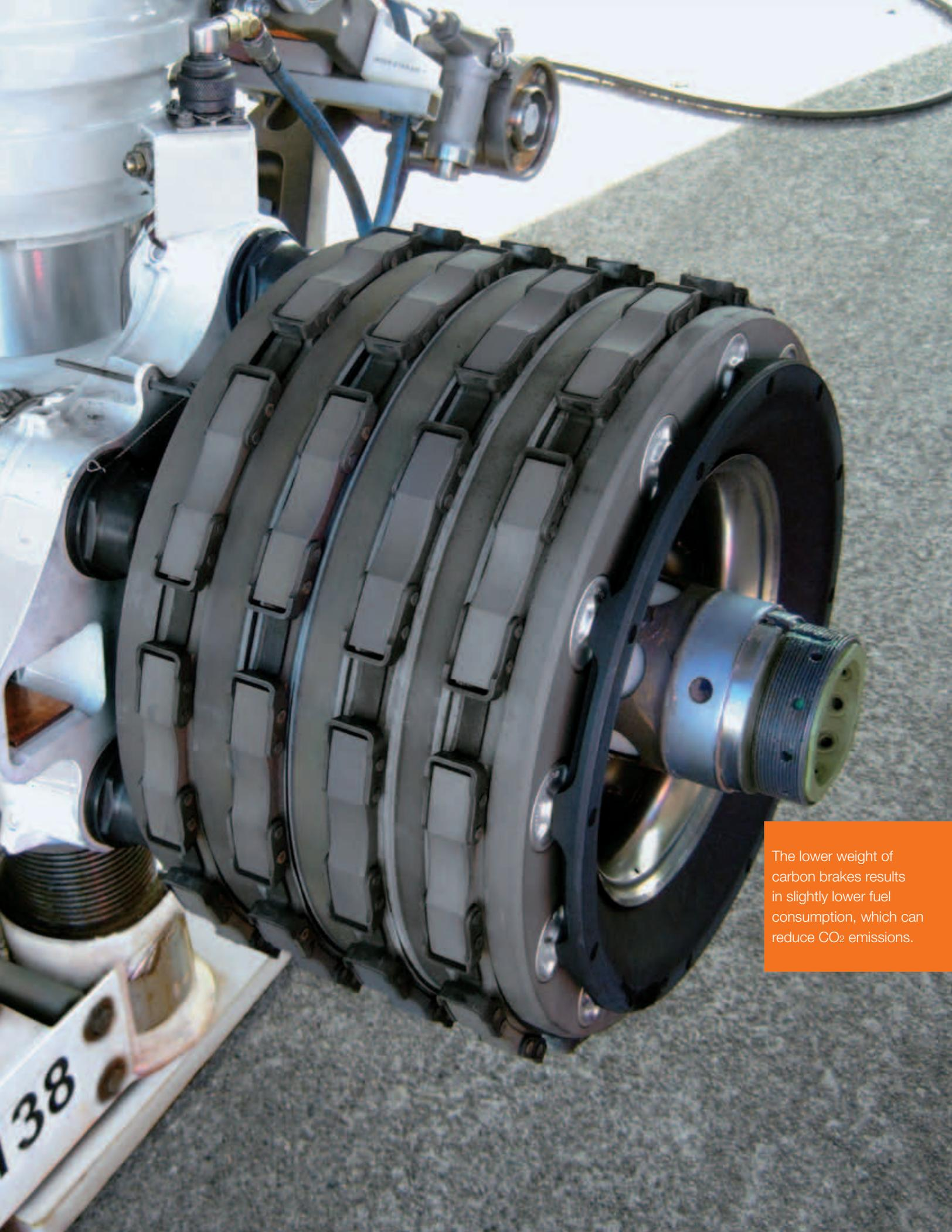
The lower weight of carbon brakes results in slightly lower fuel consumption, which can reduce CO<sub>2</sub> emissions.
