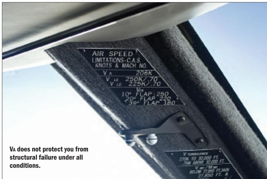
**$V_A$  does not protect you from structural failure under all conditions.**
