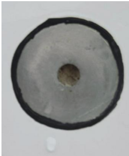
Close-up of the outflow valve static port.
