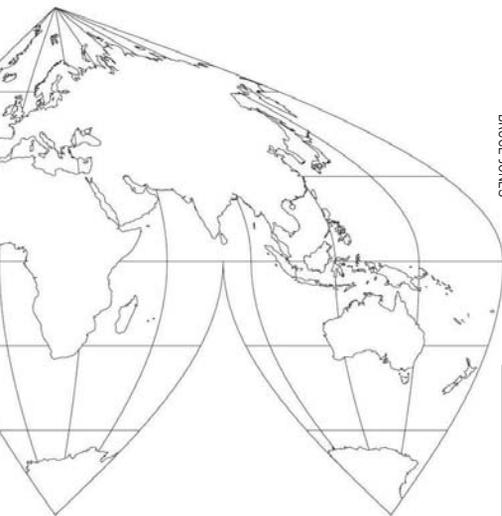
A six-point sinusoidal projection of the Earth
