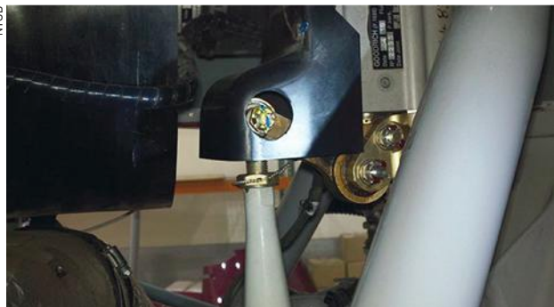
Eurocopter AS350 nut and split pin on fore/aft servo input rod
