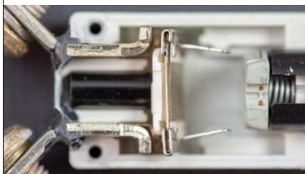
A conventional “hard” circuit breaker
