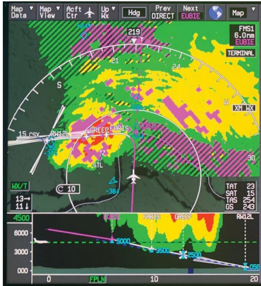
A look at the weather prior to landing, using a 3-D radar in a Gulfstream GVII-G500. Credit: Stephen Testerman
