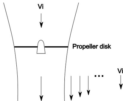
**Entrained flow: the velocity of the propeller wake is higher than the freestream velocity, and a turbulent shear layer develops that slows the flow of the propeller wake and increases the velocity of the freestream near the propeller wake**
