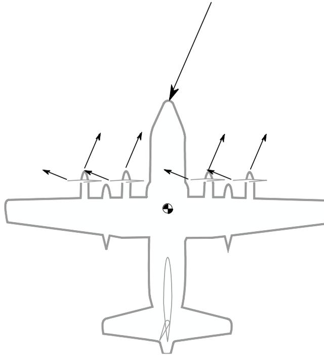
Figure 2. Propeller Normal Force in Slide Slip
