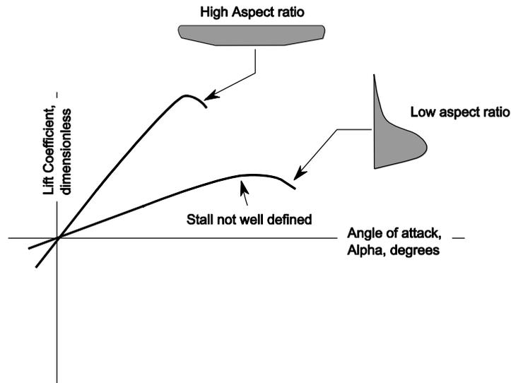
Figure 7. Rudder Angle of Attack verses Lift Coefficient
