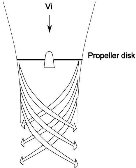
**Helical (corkscrewing) flow effect behind propellers provides a lateral velocity component above the wing to the right.**
