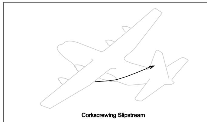
Rudder over balance has occurred at airspeeds up to 180 knots. At higher airspeeds, there is a risk of structural overload/damage/separation of the vertical stabilizer if the rudder is suddenly deflected at high side slip:
