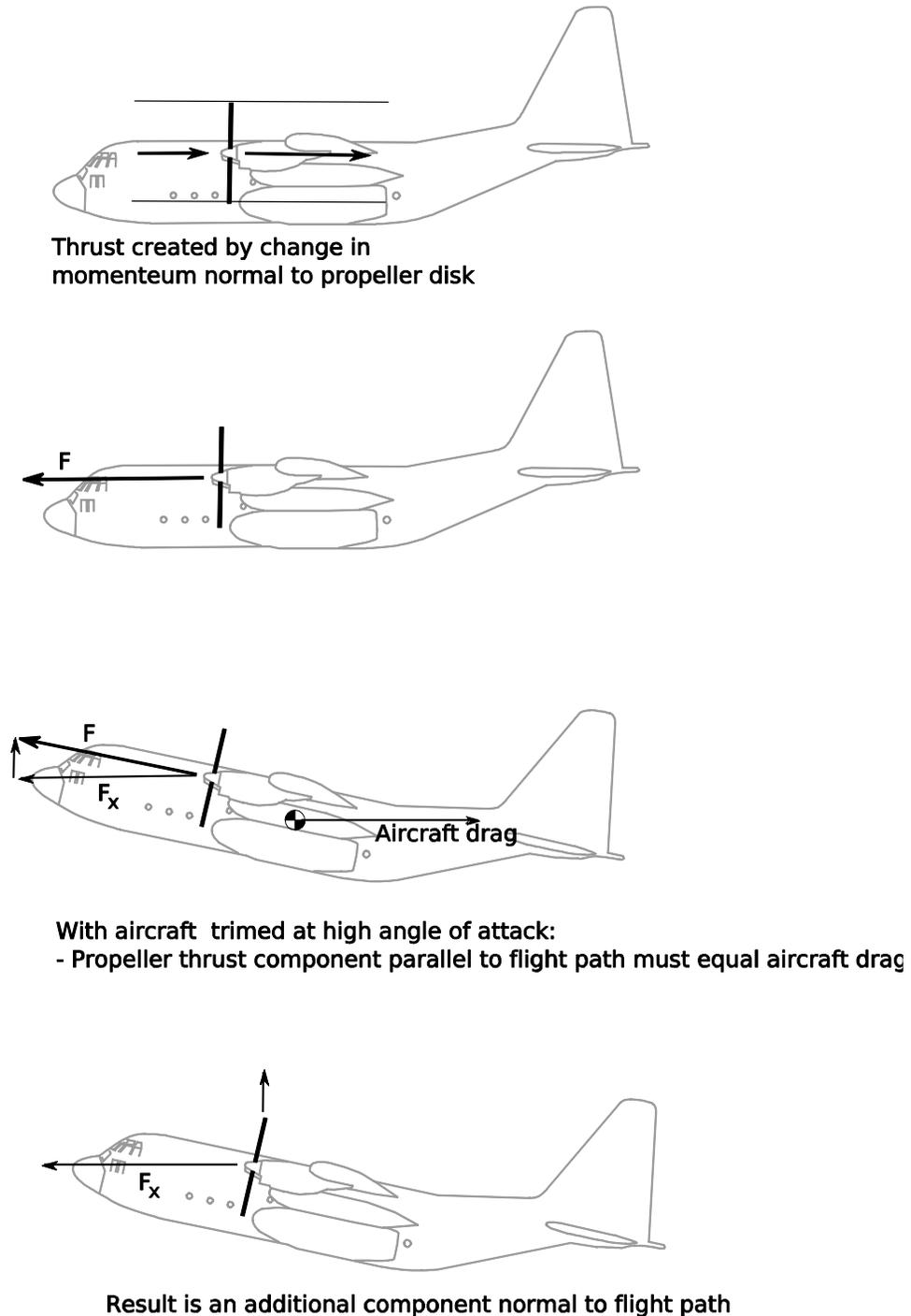
Figure 1. Propeller Normal Force due to momentum change
