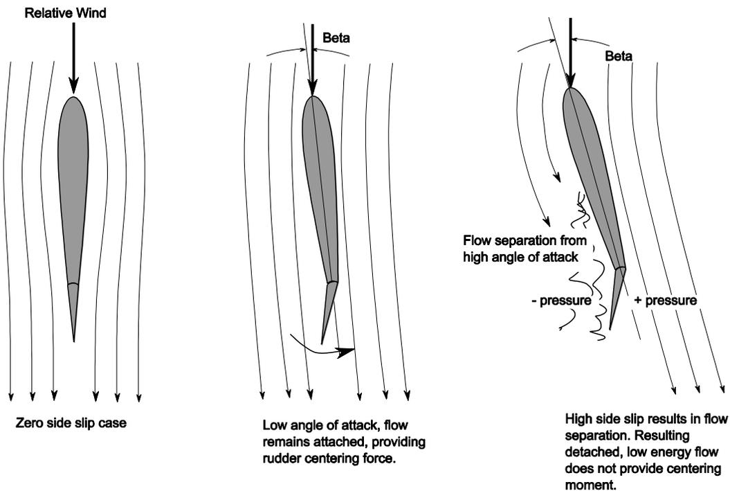
Figure 6. Rudder Force Reversal (Rudder “Overbalance”)
