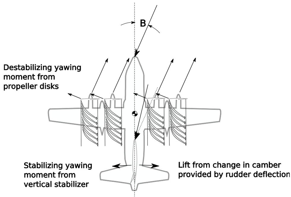
Figure 5. Reduction in directional stability at high power settings
