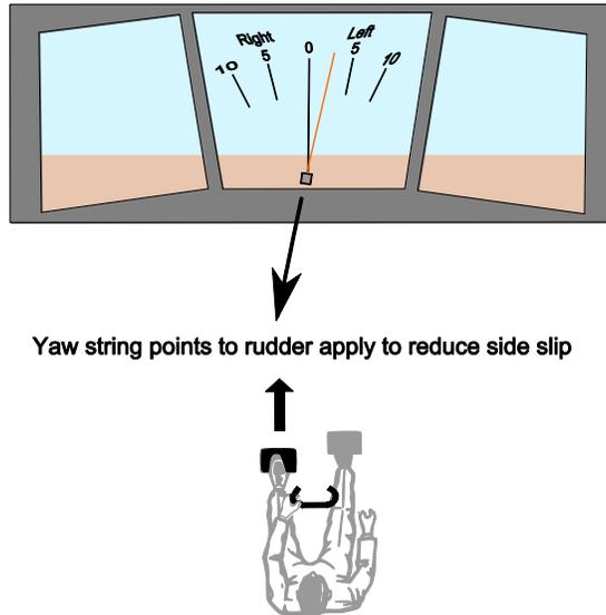
The design of the C-130 is such that high side slip angles are not accompanied by strong rolling moments from the side slip. During testing, angles of side slip as high as 40 degrees were observed without a roll off.
