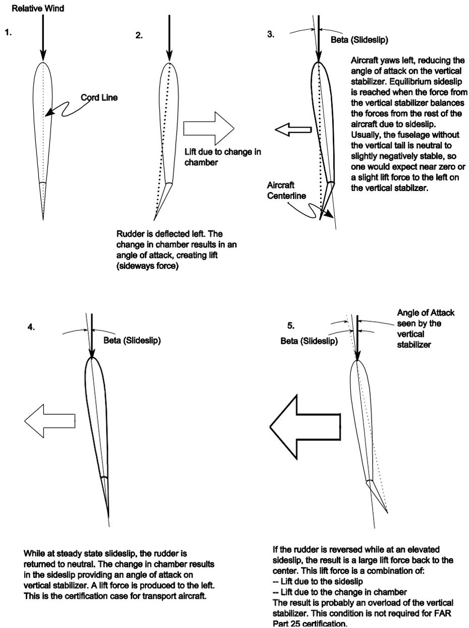
Figure 9. Possible Vertical Fin Overload with Rudder Reversal in Slide Slip
