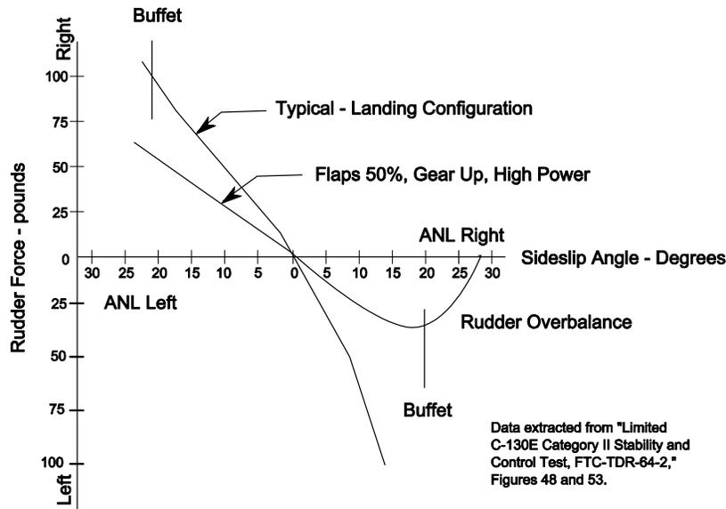
Figure 8. Rudder Force Gradient
