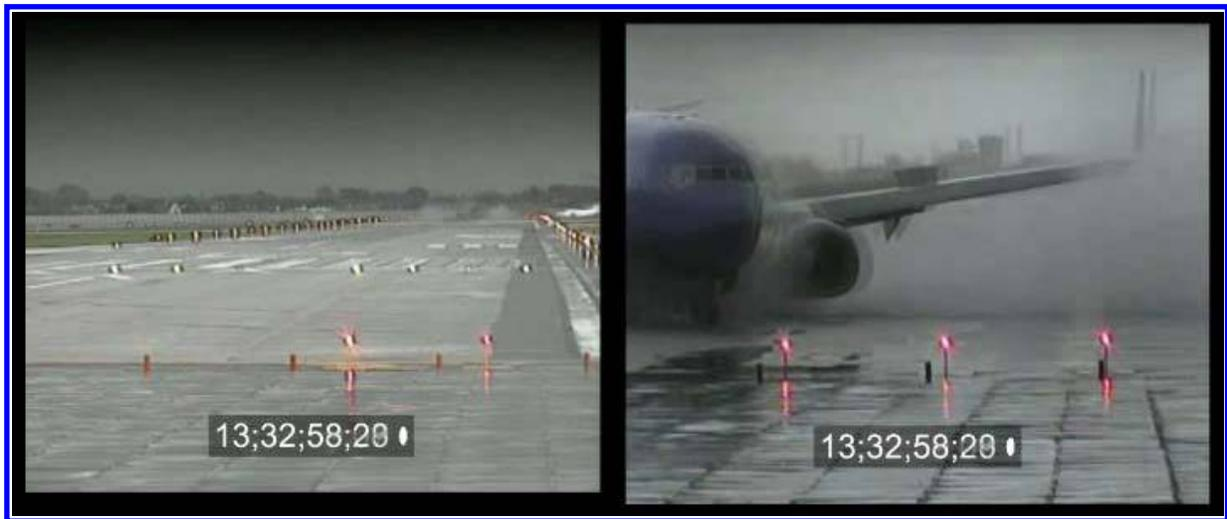
**Figure 9.** Security camera still images of Southwest Airlines flight 1919 just prior to exiting the left side near the end of runway 13C at KMDW on 4/26/2011. The view down runway 13C is shown on the left; the view down runway 31C is shown on the right.
