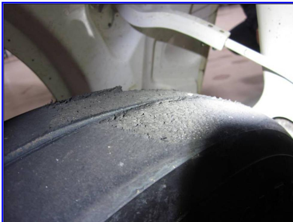
**Figure 11b.** Post-accident photo of N584JS left main gear tire, showing evidence of reverted-rubber hydroplaning (photo of right tire not available).
