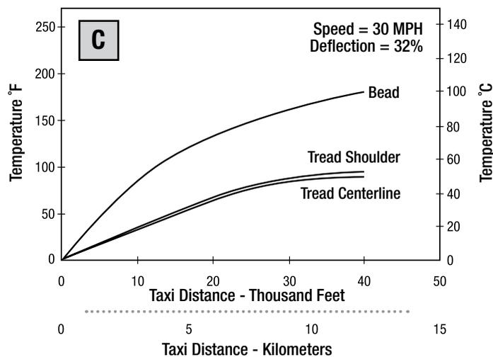
**C** Even when an aircraft tire is properly inflated and operated at moderate taxi speeds, the heat generation will always exceed the heat dissipated. (This is indicated by the ever increasing slope of the lines.) The farther the taxi distance, the hotter the tires will be at the start of the take-off.
