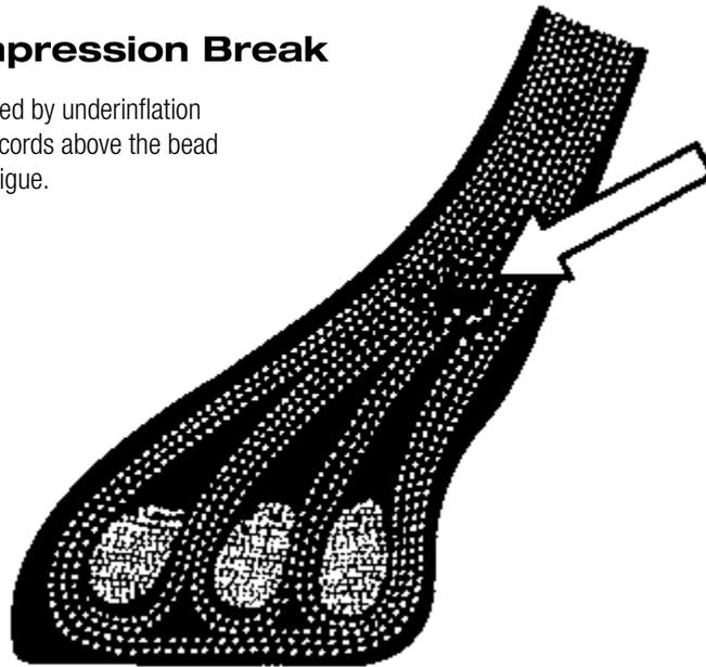
These photos show how underinflation or overloading can cause lower sidewall compression flex breaks.
