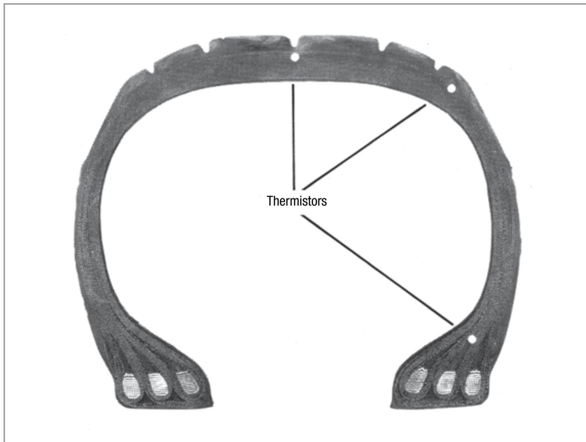
To understand the magnitude of heat generated in typical aircraft tires, several test tires were fitted with temperature sensors, or thermistors, mounted at the locations indicated. The actual temperature rise during a variety of free-rolling taxi tests was monitored and recorded. The following charts show the effect of taxi speed, inflation pressure, and taxi distance on internal heat generation for typical main landing gear tires.
