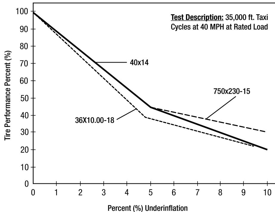
To demonstrate how rapid carcass fatigue can occur due to underinflation, the chart above shows the average of three different tire sizes run at the following conditions:
