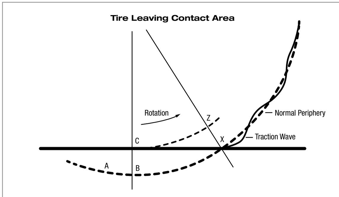
As the tire leaves the deflected area, it attempts to return to its normal shape. Due to centrifugal force and inertia, the tread surface doesn't stop at its normal periphery but overshoots, briefly distorting the tire from its natural shape. This sets up a traction wave in the tread surface.
