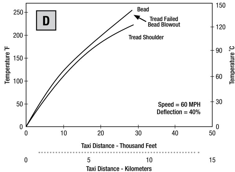
**D** This chart shows the effect of underinflation coupled with the high speed taxiing. Compare the heat generation between a tire run at 32% deflection in Chart C and this one run at 40% deflection. Not only is the slope of the 40% deflection curves much steeper (due to higher rate of heat generation) than the 32% curve, but the 40% deflection tire blew out in the lower sidewall after traveling about 30,000 feet.
