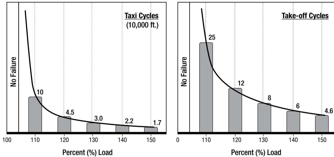
To determine if overloading has the same detrimental affect on tire life as underinflation, the same tests were run on several tires with increasing overloads. As expected, the more a tire is overloaded the quicker it fails.
