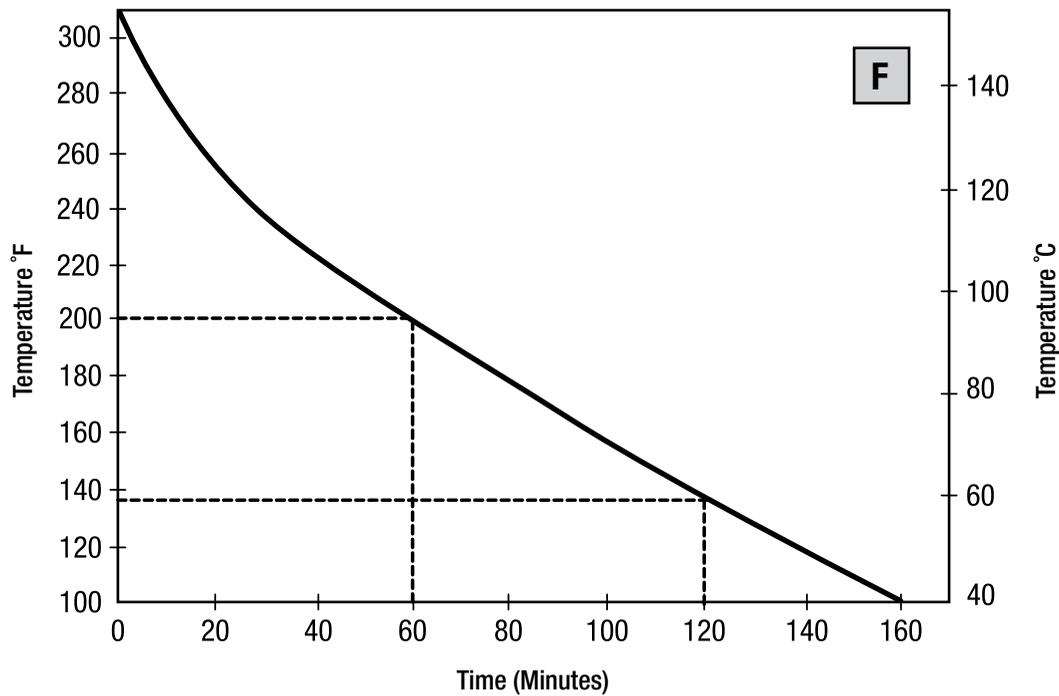
**F** On charts C and D it must be remembered that only temperature rise was indicated. Heat is cumulative. Chart F shows the time required to cool the bead area of a test tire with two fans blowing on it. This would equal approximately a 30 mph breeze. The curve indicates that the temperature in a hot tire drops 100°F in the first hour and somewhat less in subsequent hours. The cooling time of a tire mounted on an aircraft would be slightly longer due to the effect of brake temperature.
