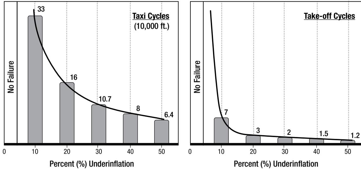
A couple of interesting findings in this study were that all the taxi cycle failures were blowouts in the lower sidewall, while the take-off cycle failures were thrown treads. From the shape of the curves we see that takeoff cycles were more sensitive to underinflation than were taxi cycles.
